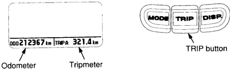
The tripmeter will show mileage in two sub modes, “TRIP A” and “TRIP B.”
