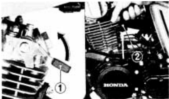
(1) Decompressor lever (2) Recoil starter
