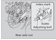
**4.** Turn both adjusting bolts an equal number of turns until the correct drive chain slack is obtained. Turn the adjusting bolts counterclockwise to tighten the chain. Turn the adjusting bolts clockwise to provide more slack.
