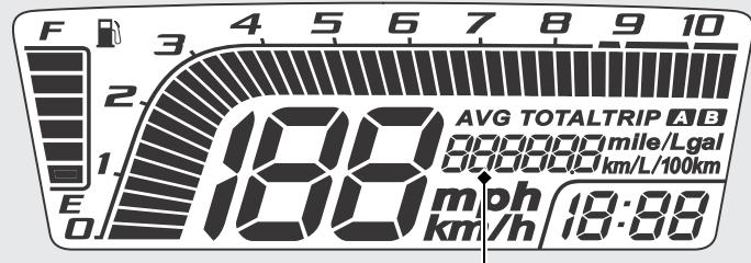
**Odometer [TOTAL] & Tripmeter [A/B] & Fuel mileage meter & Fuel consumption meter**
