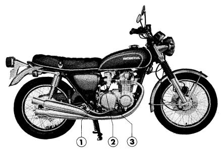
① Engine oil filler cap ② Kick starter pedal ③ Rear brake pedal
