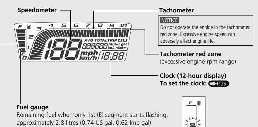
If the fuel gauge indicators repeat flashing or turned off: P.87
