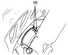
Position the lug on the speedometer gear box against the lug (8) on the left fork leg. Tighten the axle bolt to the specified torque. Front axle torque:
