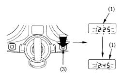
When the ignition switch is turned OFF while set the clock in the adjust mode, the time will be fixed as just before the ignition OFF.
