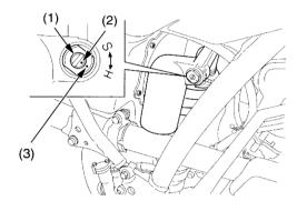
(1) compression damping adjuster(3) reference mark(2) punch mark
