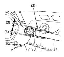
5. Measure a section of the drive chain to determine whether the chain is worn beyond its service limit. Remove the drive chain and measure the distance between a span of pins from pin center to pin center. If the distance exceeds the service limit, the chain is worn out and should be replaced.
