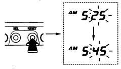
6. To end the adjustment, push the SEL button or turn the ignition switch OFF. The display will stop flashing automatically and the adjustment will be cancelled if the button is not pushed for about 2 minutes.
