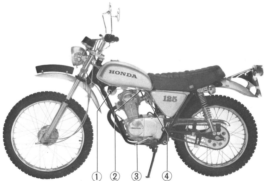
① Main switch ② Fuel valve ③ Gear change pedal ④ Choke lever
