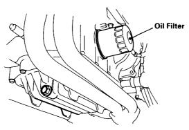
3. Apply a thin coat of engine oil to the rubber seal on the new oil filter.
