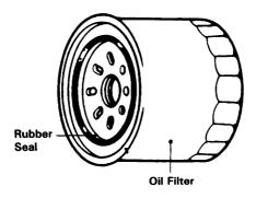
4. Using a special tool and a torque wrench, install the new oil filter and tighten it to the specified torque:
