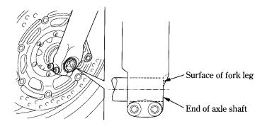
Install the bolts and tighten to the specified torque: axle bolt:
