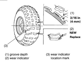
To check the condition of a tire tread, measure the groove depth (1) in the center of the tire, or check the wear indicator (2).
