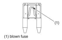
The fuse is located in the battery compartment.
