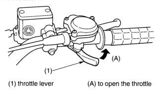
The throttle controls rpm (speed). To increase engine rpm, press the lever (1) with your thumb. To reduce engine rpm, release pressure on the lever. The throttle will automatically return to the closed position (engine idle) when you remove your thumb.
