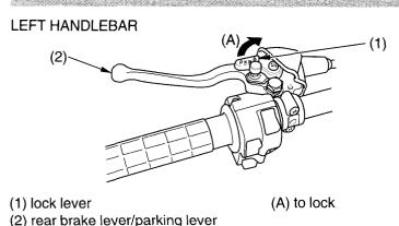
The lock lever (1) on the rear brake lever (2) allows it to be used as a parking brake. To operate, first squeeze the rear brake lever using your left hand and then lock it with the lock lever using your right hand. See *Parking* page 81.
