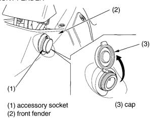
The accessory socket (1) is attached to the left side of the front fender (2). You can use the accessory socket to power a trouble light, spotlight, CB radio, or cell phone, etc.
