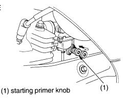
The starting primer knob (1) is located on the carburetor float bowl. The knob may be used when starting the engine in extremely cold weather ( $-15^{\circ}$ C,  $5^{\circ}$ F). See *Starting Procedure*, page 61.
