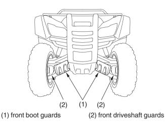
Check the front boot guards (1) and front driveshaft guards (2) for cracks, damage or looseness.
