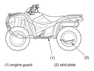
The engine guard (1) protects the frame and engine crankcase. The skid plate (2) protects the rear final gear case. Check the guard and plate for cracks, damage or looseness at intervals shown in the Maintenance Schedule.
