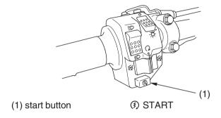
The start button (1) is used for starting the engine. Pushing the button in starts the engine. See *Starting Procedure*, page 50.
