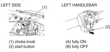
1. Pull the choke knob (1) left all the way to fully ON (A) position, if the engine is cold.
