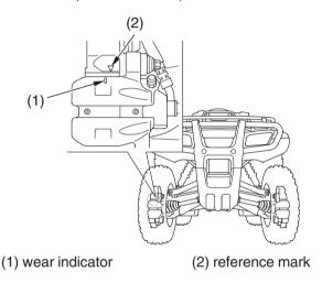
Check the wear indicator (1). Remove the front wheels (page 196). If the wear indicator aligns with the reference mark (2), both pads must be replaced, see your Honda dealer for this replacement.
