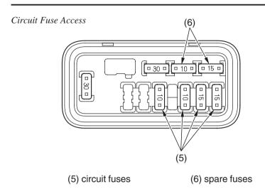
1. To check or replace a circuit fuse (5), pull the old fuse out of its retaining clips.
