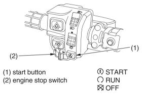
The start button (1) is used for starting the engine. Pushing the button in starts the engine. See *Starting Procedure*, page 67.
