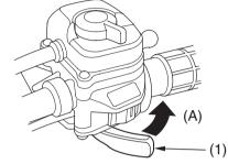
(1) throttle lever(A) to open the throttle
