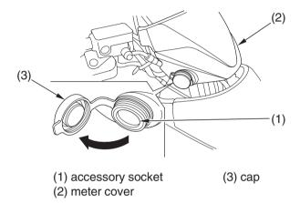
The accessory socket (1) is attached to the right side of the meter cover (2). You can use the accessory socket to power a trouble light, spotlight, CB radio, or cell phone, etc.
