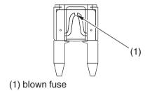
The main fuse and the circuit fuses are located in the battery compartment.
