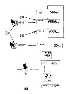
(3) Tripmeter A (4) Tripmeter B
