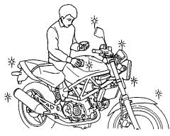
Dry and lubricate any moving parts that may be affected by water.
