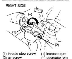
The engine must be at normal operating temperature for accurate idle speed adjustment. Support the motorcycle
