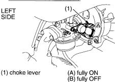
1. Pull the choke lever (1) up all the way to fully ON (A).
