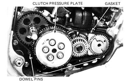
Remove the clutch lifter, steel ball.
