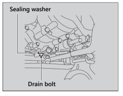
**6.** Install a new sealing washer onto the drain bolt. Tighten the drain bolt.
