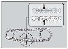
**5.** Rotate the rear wheel and check that the chain moves smoothly.
