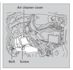
**4.** Remove the screws and air cleaner housing cover.
