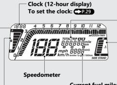
Odometer [TOTAL] & Tripmeter [TRIP A/B] & Stopwatch \( \bigstyle{\textit{P}}\)P.20
