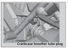
**3.** Reinstall the crankcase breather tube plug.
