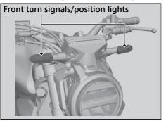
The front turn signals/position lights use several LEDs.
