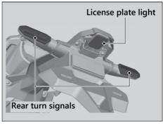
The license plate light uses a LED. The rear turn signals use several LEDs. If there is an LED which is not turned on, see your dealer for servicing.
