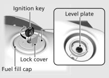
Do not fill with fuel above the level plate. Fuel type: Unleaded gasoline only Recommended fuel octane number: Pump Octane Number (PON) 86 or higher. Tank capacity: 4.15 US gal (15.7 liters)
