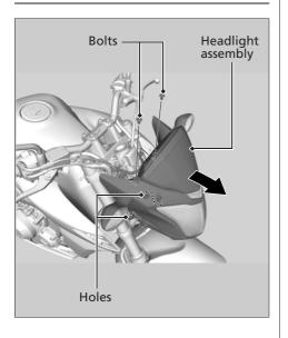
When removing and installing the headlight assembly, be careful not to damage the wire harness.
