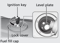
Do not fill with fuel above the level plate. Fuel type: Unleaded gasoline only Recommended fuel octane number: Pump Octane Number (PON) 86 or higher. **Tank capacity:** 4.41 US gal (16.7 liters)
