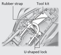
The U-shaped lock is held in place under the seat.
