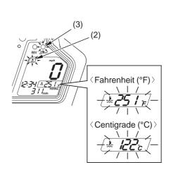
(2) high coolant temperature indicator(3) warning indicator
