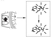
6. To end the adjustment, press control button B or turn the ignition switch OFF. The display will stop blinking automatically and the adjustment will be cancelled if the button is not pressed for about 30 seconds.
