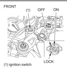
To unlock the steering lock, insert and push down on the key and turn it to the right to the OFF position.
