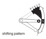
Your motorcycle has six forward gears in a one-down, five-up shift pattern which is coordinated with a cable-operated clutch system.
