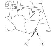
(1) engine oil drain bolt(2) sealing washer
